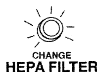
Fig. 3: HEPA Filter Change Light
